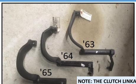
NOTE: THE CLUTCH LINKAGE PIN IS ON THE LEFT ON '63/'64 AND IS ON THE RIGHT (TOWARDS ENGINE) ON THE '65.
