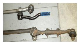
63 & 64 Falcons (sometimes called the Mustang conversion). This conversion eliminates most of the bump steer found in the earlier Falcons. NOTE: The Falcon can not use the Mustang center link. You must use a 1965 Falcon center link.
