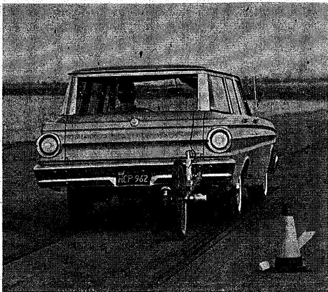
Extra weight didn't make much difference in Falcon's stopping distance—only six feet longer from 60 mph when fully loaded.
